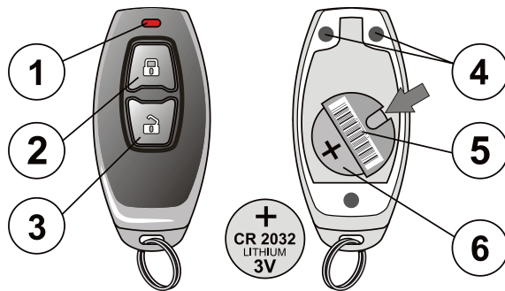
Figure: 1 – LED indicator; 2 – setting (ON) button; 3 – unsetting (OFF) button; 4 – bottom cover screws; 5 – production code; 6 – CR2032 battery (remove the battery by pressing it in the direction of the arrow).
